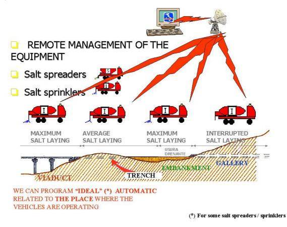
full-scale winter operations, for each of vehicles in order to distribute the correct quantities on viaducts, fasticing shadowed areas, areas with drainage pavements and similar (dosages, type of salt (dray or humid) according to a predetermined programme<sup>3</sup>.
