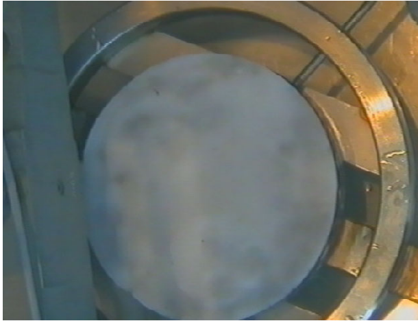
Figure 4: Continuous surface layer of hydrohalite on pavement sample, SMA+Hydrohalite (g)
