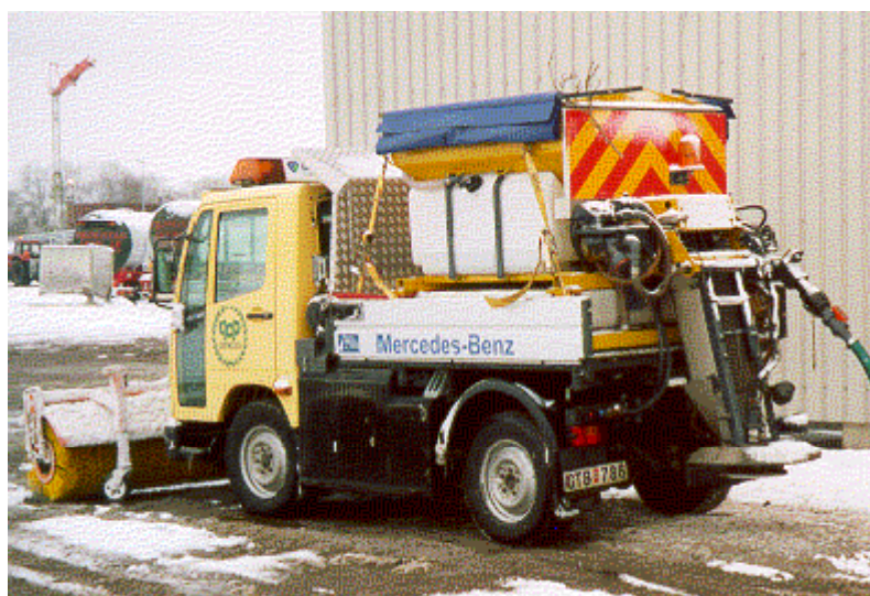
Figure 1. The Mercedes Benz UX 100 Used in the Large-scale Study, Equipped with a Front-mounted Broom for Snow Clearance and a Spinner for Spreading Brine, or Pre-wetted Salt.
