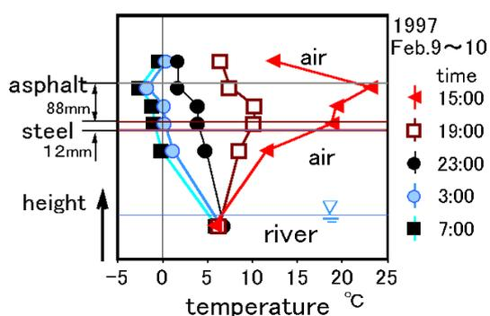
Fig.19 Change of temperatures at various points on a steel deck bridge
