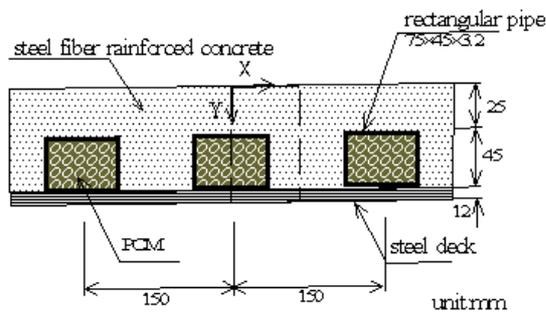
**Fig. 23 Section of steel deck with PCM**
