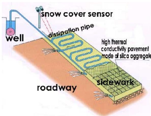
Fig.1 Outline of cascade SMS using underground water
