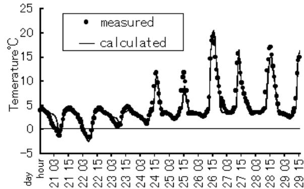
**Fig.28 PCM temperatures on steel deck bridge**
