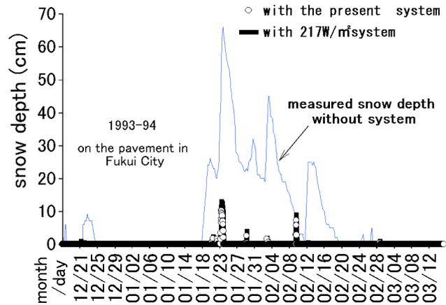
Fig.10 Result of snow melting simulation
