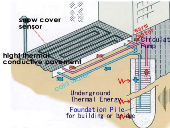
**Fig.4 Outline of SMS using underground thermal energy collected by foundation piles**
