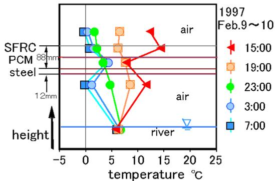
**Fig.21 Change of temperature at various points of steel deck bridge with PCM**
