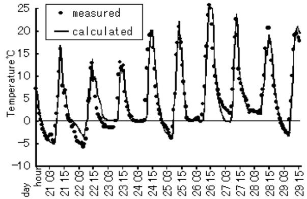
**Fig.26 Road surface temperatures on steel deck bridge without PCM**
