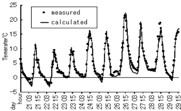
**Fig.27 Road surface temperatures on steel deck bridge with PCM**
