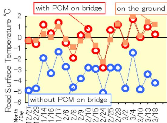
**Fig. 24 Daily minimum road surface temperatures**
