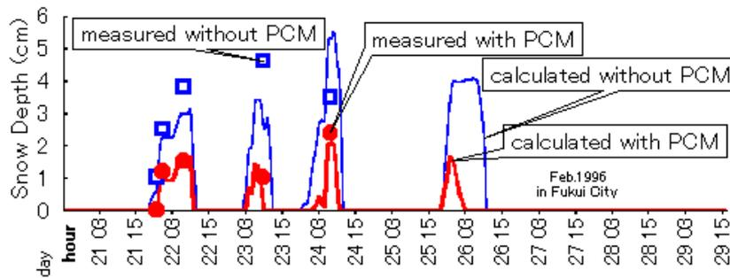
**Fig. 29 Snow depth on steel deck bridge with and without PCM**
