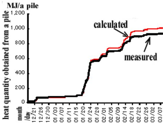
Fig.9 Heat quantity obtained from a pile
