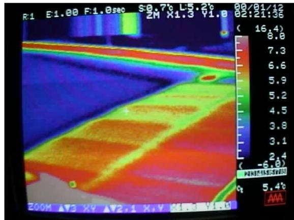
**Photo. 6** Isothermal contour of pavement connected to RHCS and BHES (Jan. 12, 2000)
