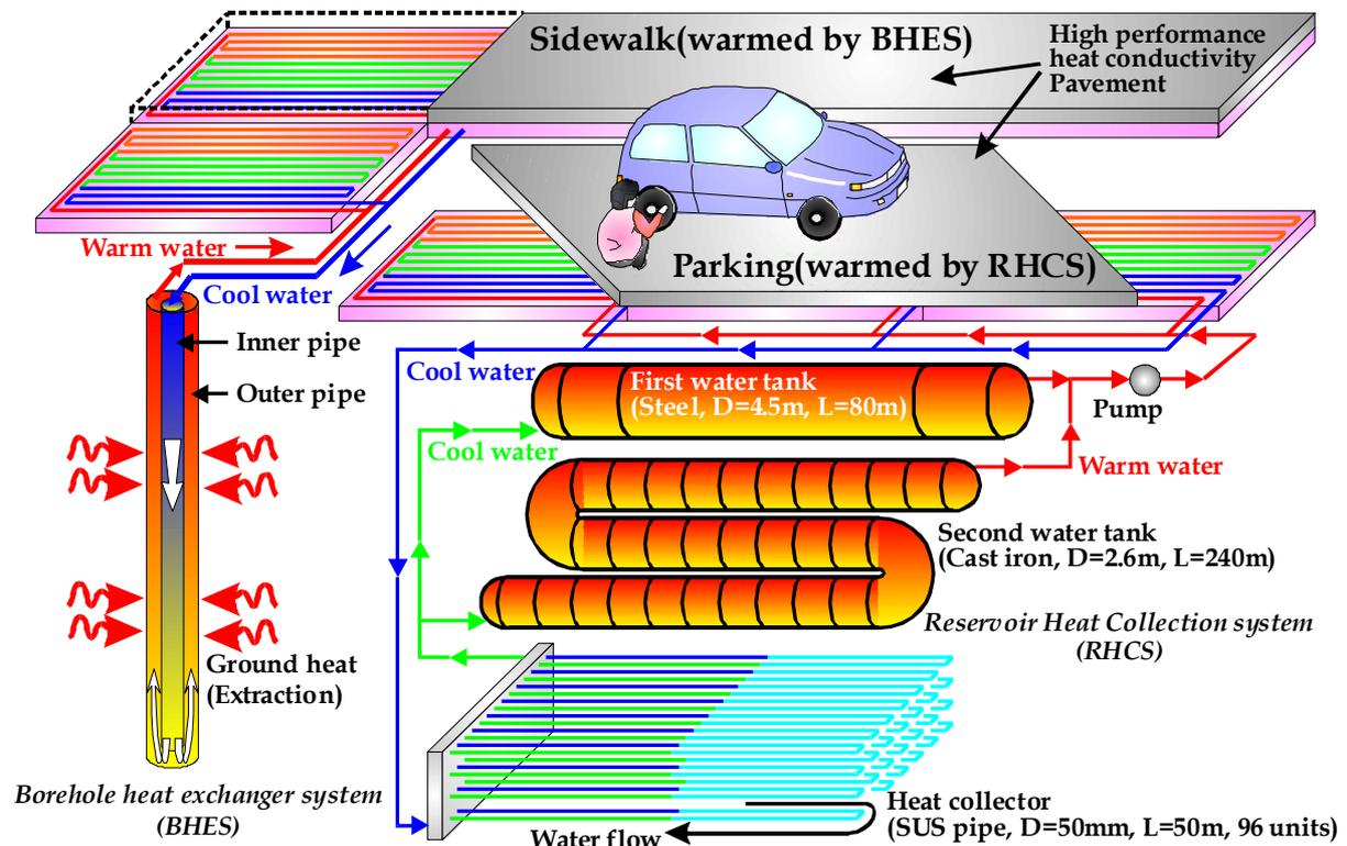
Figure 1 Schematic view of snow melting systems using ground heat at "HACHI-KITA"
