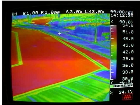
**Photo. 2** Isothermal contour of pavement connected to RHCS and BHES (14:12, Aug. 3, 1999)
