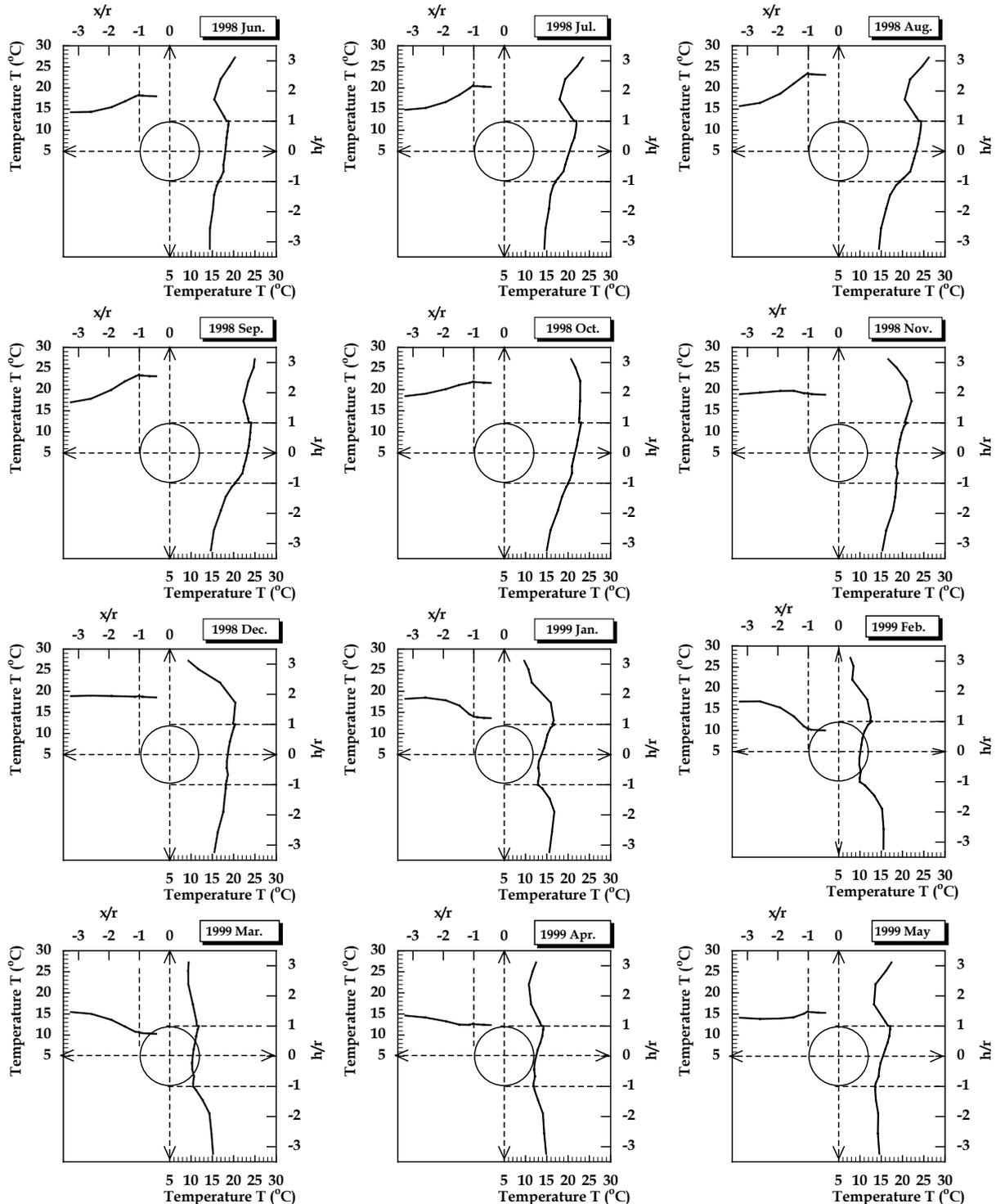
Figure 3 Temperature profiles of tank water and the surrounding ground from June, 1998 to May, 1999
