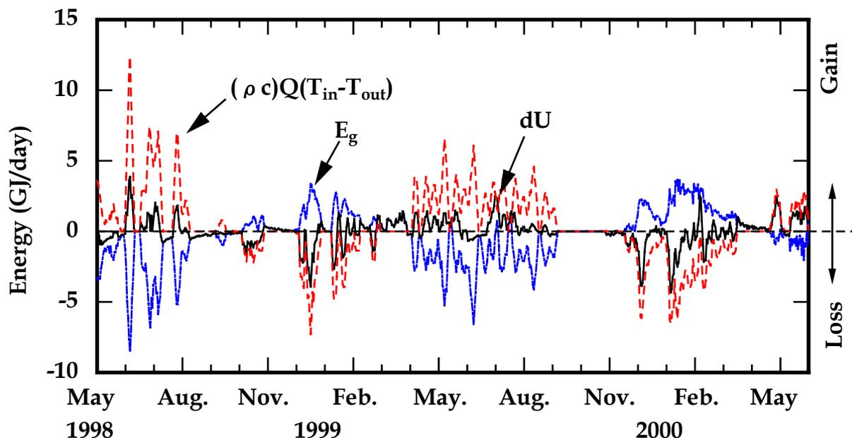
Figure 4 Time series of heat energy balance of the first water tank from May 1998 to Jun., 2000
