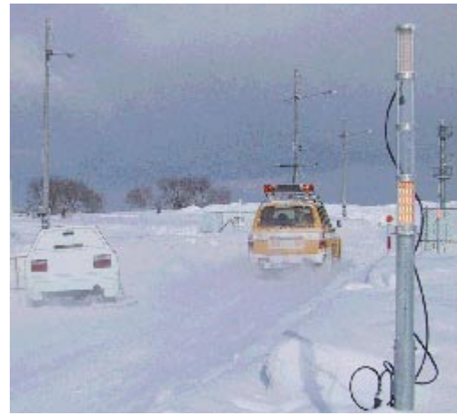
Figure 6 Driving Experiment: At left is a panel simulating the obstacle; at right is the experimental light emitting delineator.
