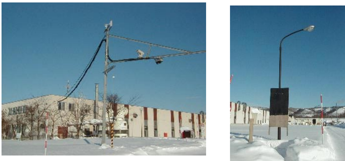
Fig. 8 CCD camera and backdrop plate
