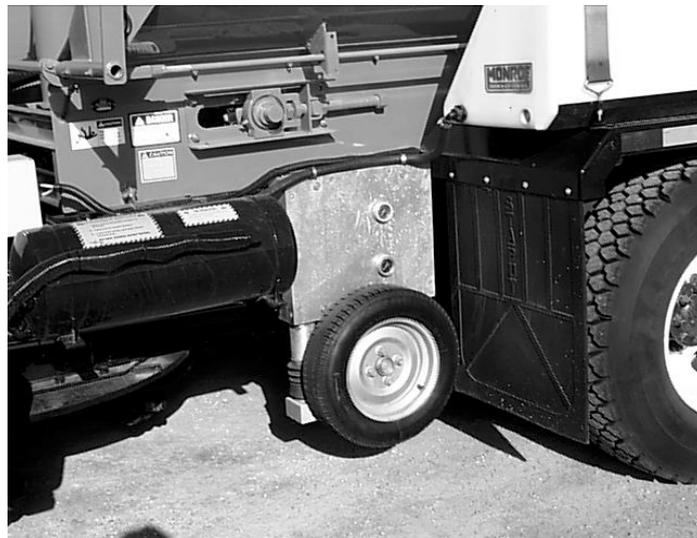
**Figure 4. SALTAR Friction Measuring Device Mounted on a Salt/plow Truck**
