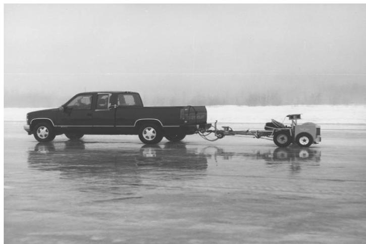
**Figure 1 ROAR Friction Trailer**
