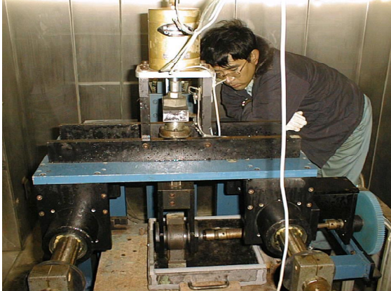
Photo 5 View of fracture test of ice-board
