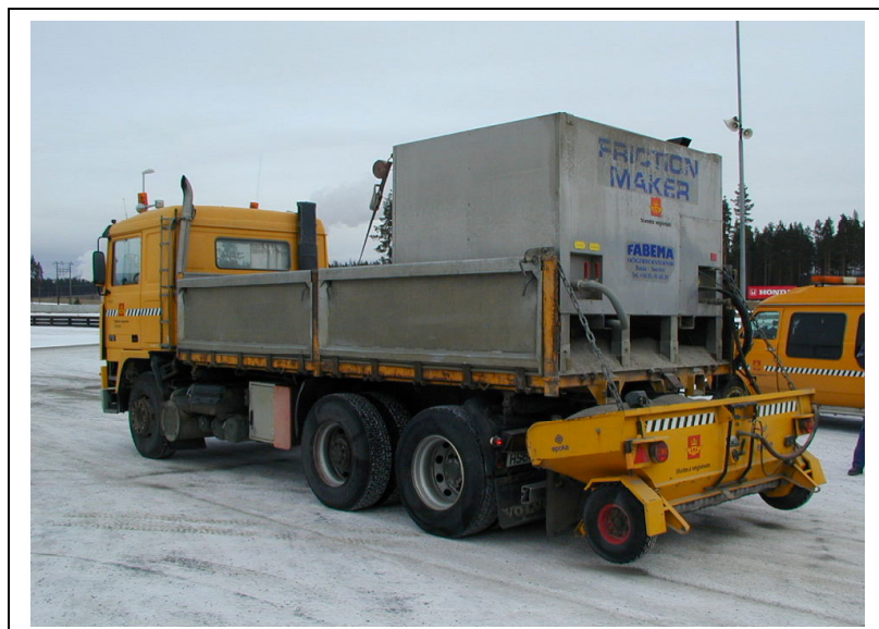
FIGURE 1 Swedish Prototype for Warm Wetted Sand.
