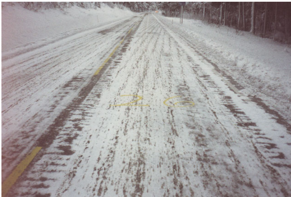
Figure 13 Test Field strewn with Warm Wetted Sand 18 th January 2001. Picture taken 22 nd January.
