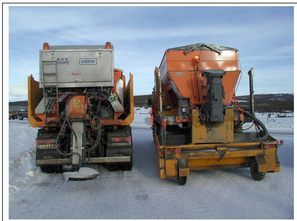
FIGURE 5 New Concept for Warm Wetted Sand. The Truck to the left can also be used for spreading Salt.
