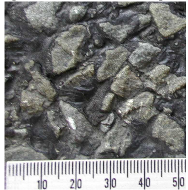
Sample 4: Untrafficked Grade 5 Chipseal (9mm nominal aggregate size), MPD = 1.88mm
