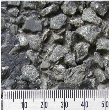
Sample 2: Untrafficked Grade 3 Chipseal (16mm nominal aggregate size), MPD = 2.15mm
