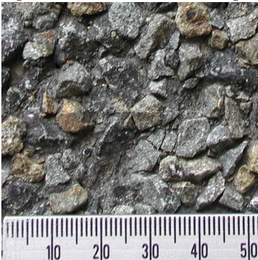
Sample 4: Untrafficked Grade 5 Chipseal (9mm nominal aggregate size), MPD = 1.88mm
