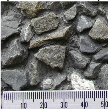
Sample 3: Trafficked Grade 3 Chipseal (16mm nominal aggregate size), MPD = 1.08mm
