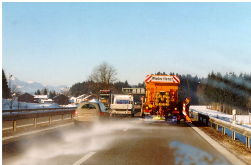
Figure 12: Application of dry salt (fine grain saline salt, approx. 30 g/m 2 at approx. 50 km/h)
