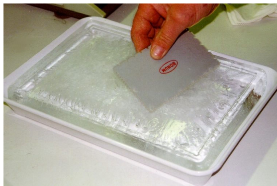
Figure 9: Distribution of prewetted salt on ice slab with toothed spatula
