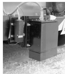
Photo 14 Measurement of road surface skid resistance coefficient
