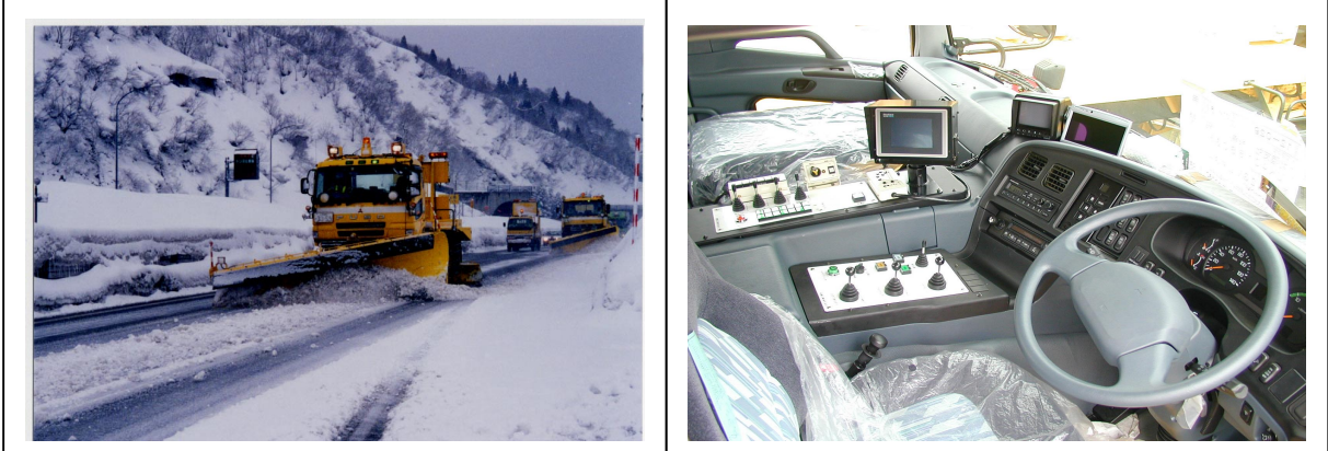
Fig. 6 One-operator snow removal truck (external and internal views)
