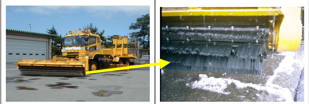
Fig. 7 Slush-removal truck and front brush
