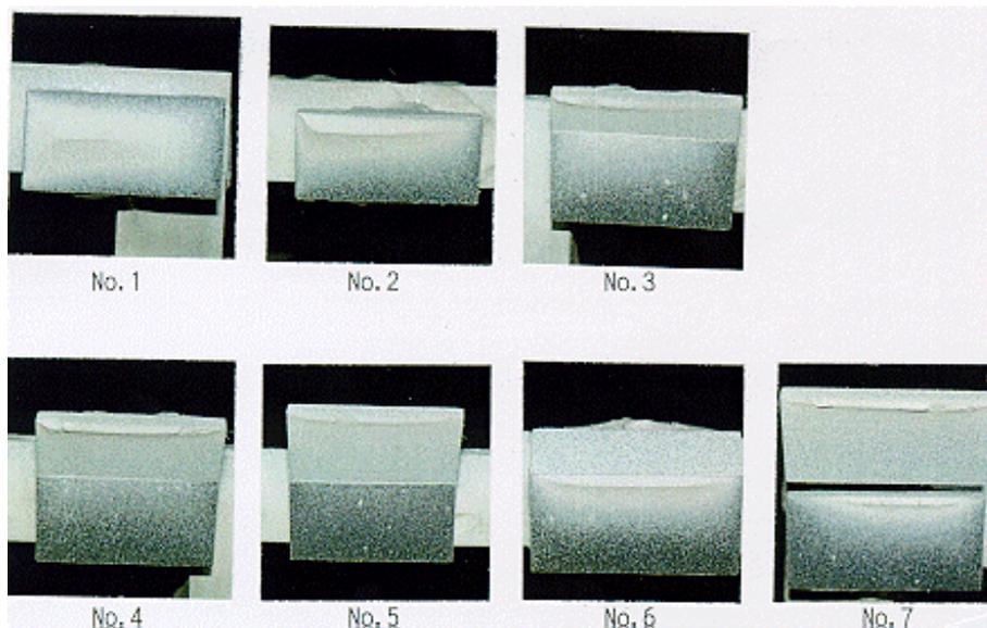
**Photo 4 Snow Accretion in the Wind Tunnel Test**
