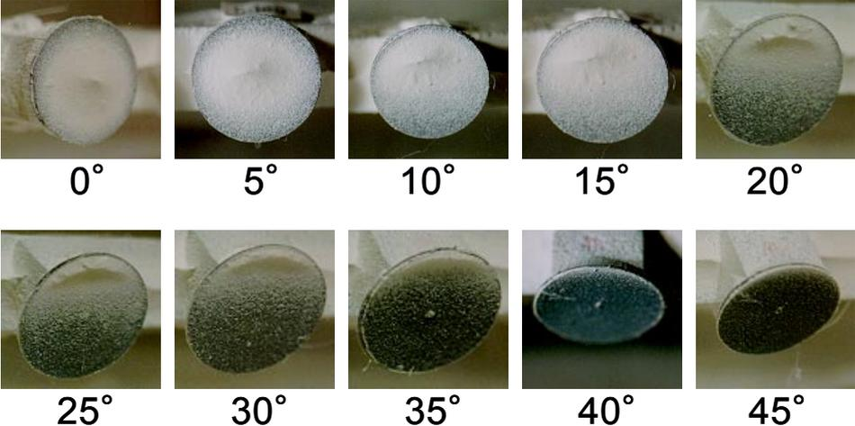
**Photo 1 Snow Accretion in the Wind Tunnel Experiment**
