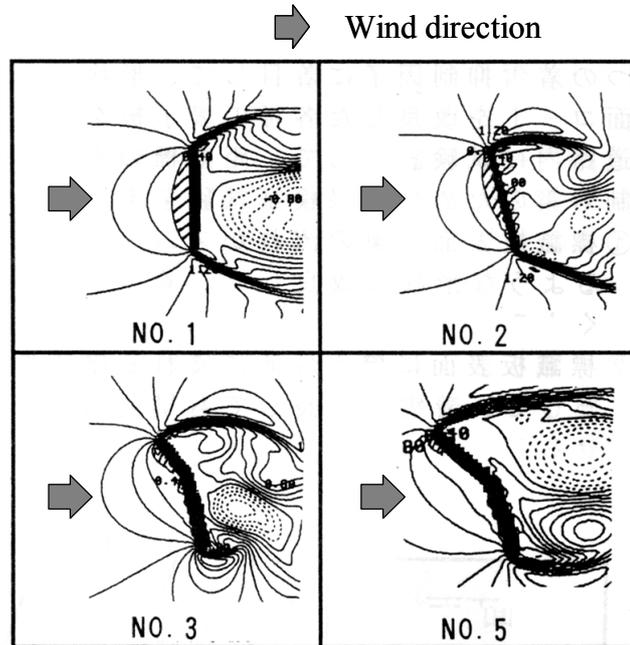
**Figure 4 Equivalent Wind Velocity Rate Diagrams**
