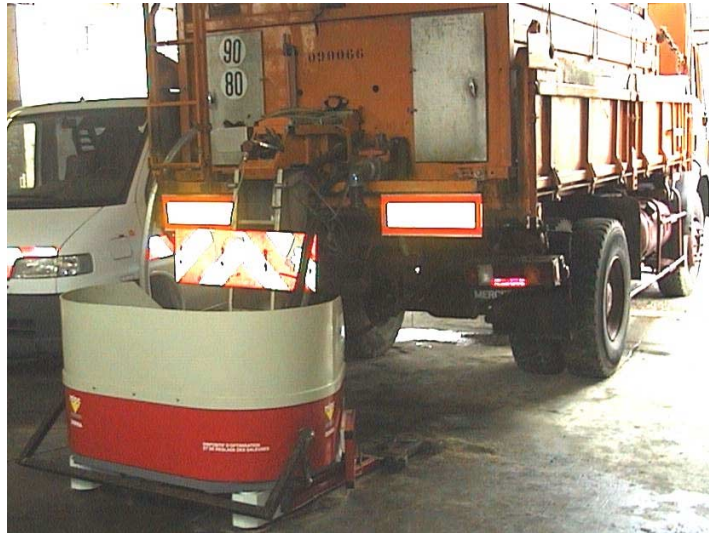
Fig. 8: Spreading rate measurement with DORSA
