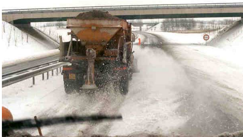
Fig. 4: Spreading de-icing agent on melting wet snow
