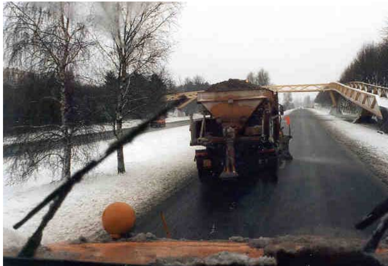
Fig. 3: Road scraping and treatment on a suburban ring road
