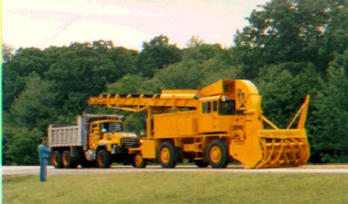
Figure 4: Single-Lane Obstructing Rotary Snowplow (Photo Courtesy of Pennsylvania Department of Transportation)
