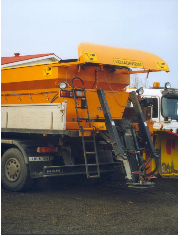
Figure 6. Winter maintenance truck with spoiler to prevent deposits of snow on the salt spreading disc. (Photo Thordarson)
