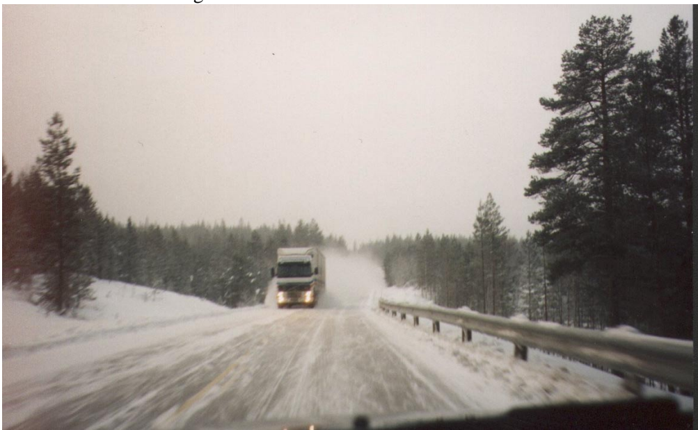
Figure 1. Photo of a meeting truck showing that the generated snow cloud reduces the visibility to almost zero in the rear of the truck. (Photo courtesy: Dagfinn Moe, SINTEF, Trondheim)
