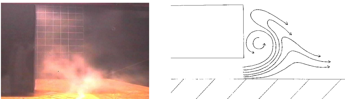
Figure 7. Results of the tests with no spoiler. Photo and the assumed streamlines. (Maelum 2000)
