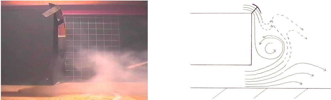
Figure 8 Results of the tests with spoiler on top and rear. Photo and the assumed streamlines. The broken lines represent weak airflows. (Mælum 2000)
