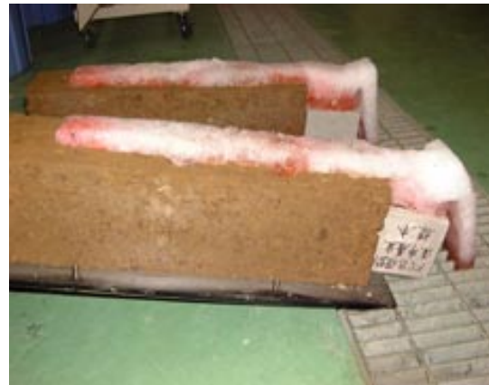
Figure 15 B test with different slope angles (foreground: 10 deg., background: 5 deg.)
