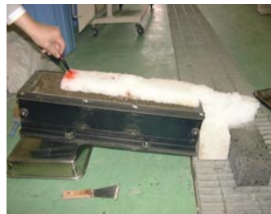
Figure 16 Snowmelt test on sand
