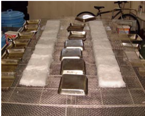
Figure 5 Snow-on-wire-netting test (before test)
