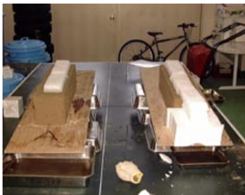
Figure 9 Snowmelt test using soil specimen (left: A test, right: B test)
