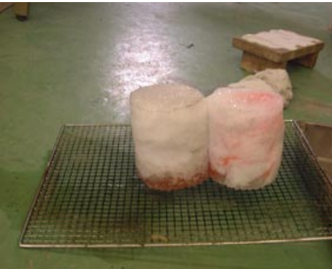
Figure 4 Meltwater dripping from lowest point of snow block
