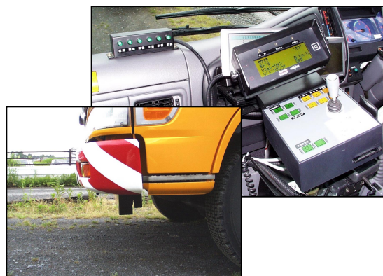
Photo 2 Operation control panel (above) and road surface judgment sensors (below)
