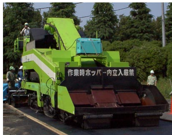
Figure 5.3 Multi-asphalt Paver (MAP)
