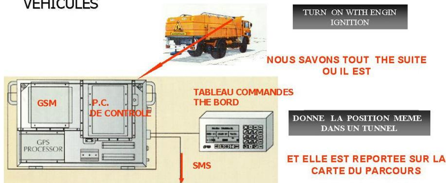
LA POSITION EST RELEVÉE PAR AU MOINS DEUX SATELLITES ET LA CORRECTION DE POSITION EST FAITE AVEC UNE PRÉCISION DE QUELQUES MÈTRES, SUFFISANTE POUR LES BUTS DU SYSTÈME
