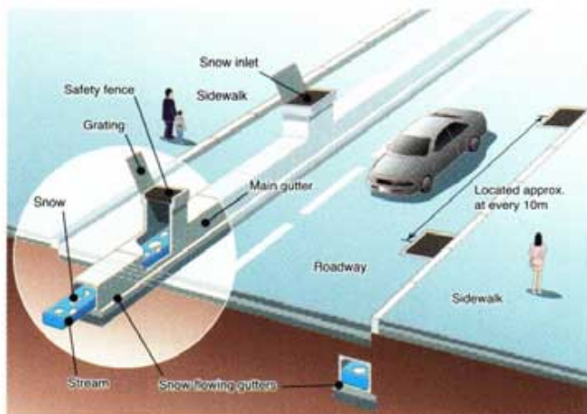
Heat sources of snow-flowing tanks 1) processed sewage that already carries heat to melt snow, and 2) residual heat from incineration plants, etc.
