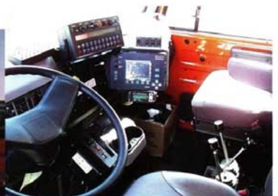
Interior view of the Concept Vehicle, showing application controller and mobile data terminal
